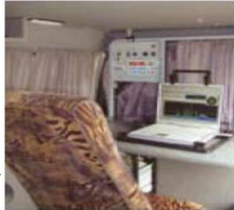
Operator console to manage jamming
